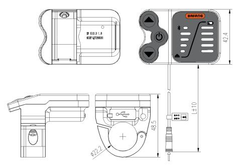
Housing material is ABS, decal material is PC with UV-Resistance.
